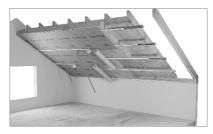
2. Further vapour control layer strips should be installed with a suitable overlap, which is printed on the membrane and bonded with single-sided (e.g. Corotop FIX) or double-sided tape (e.g. Corotop MIX).
